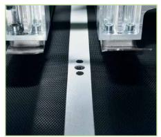
After finishing the folding process, pieces are stacked on a dedicated stacker station. As a standard, the **T.towel** is provided with 3 stacker stations, optionally a 4th stacker station is possible as well as a stacker with a different width.
