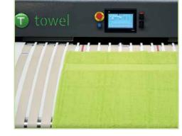
The T.towel is provided with a special feature to fold pieces that need extra corrections before being folded, like fitted sheets. After placing the sheet on the feeding table and pushing the button, the piece runs inside the machine and makes an automatic stop for correcting the tail end of the piece. Then, the operator pushes the button a second time so the folding process can start.
